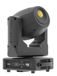
**Pixie** Spot was the first TRIBE spot moving head to deliver a full spectrum chromatic synthesis, equipped with a 60W RGBW/FC LED light source to perform limitless brightness, intense and saturated colours as well as proper whites. **Pixie** Spot can be also controlled wireless through the optional USB Wi-Fi transceiver in combination with WIFIBOX and the SmartColor app.
