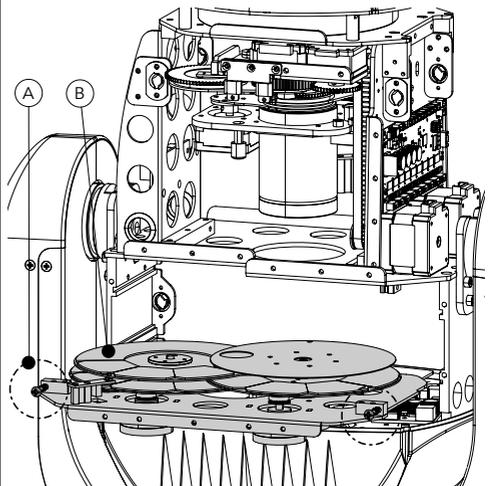
To remove the Colors and Fixed Gobo wheels module:
