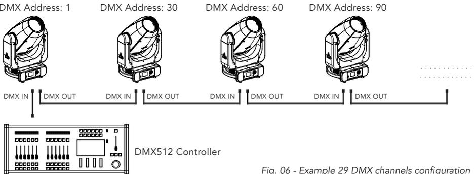
Fig. 06 - Example 29 DMX channels configuration
