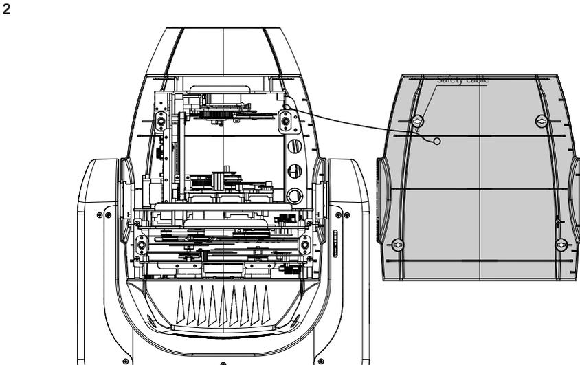
Unclip the safety cable on both sides (2).
