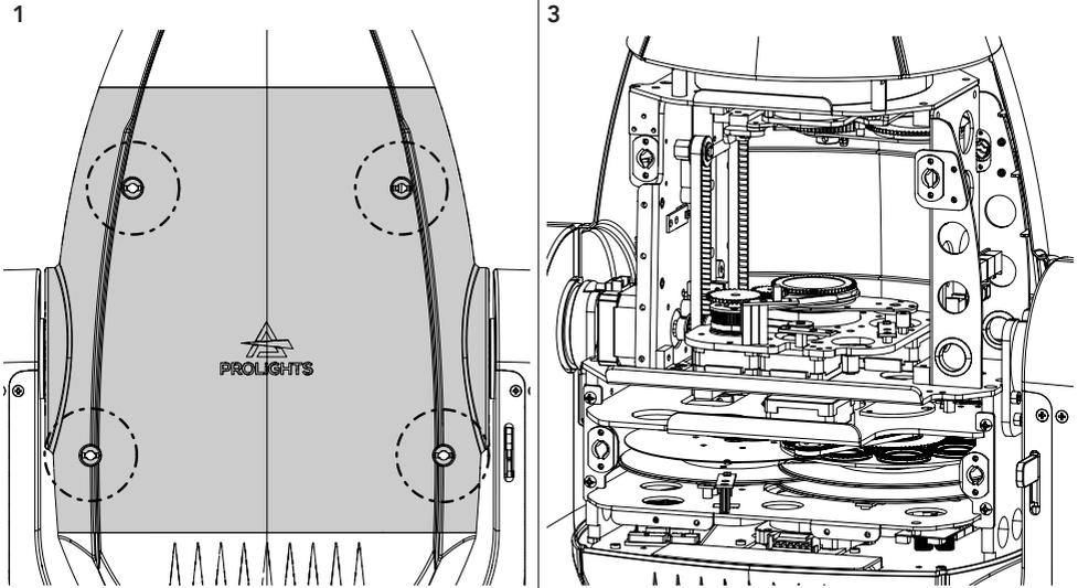
Before removing rear cover, place the head in a horizontal position and engage both the PAN and TILT locks for added stability. See the "PAN AND TILT LOCK" paragraph (pag. 6). Loosen and remove the marked screws and opening the head covers (1) from both sides.
