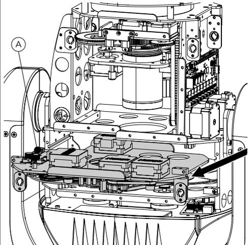
To remove the Animation and Gobo wheels module, open the head covers (see section "PERIODIC CLEANING") and proceed as follows:
