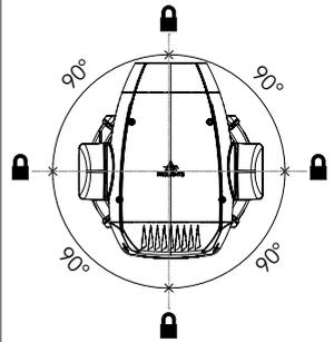
TILT Mechanism lock and release
